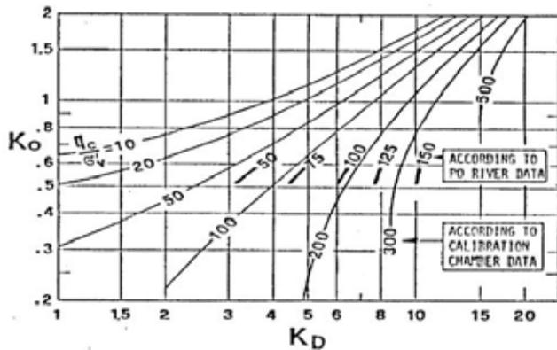
Figure 5. Chart for estimating  $K_o$  in sands as a function of DMT  $K_D$  and CPT  $q_c/\sigma'_{v0}$  (After Marchetti, 1985)
