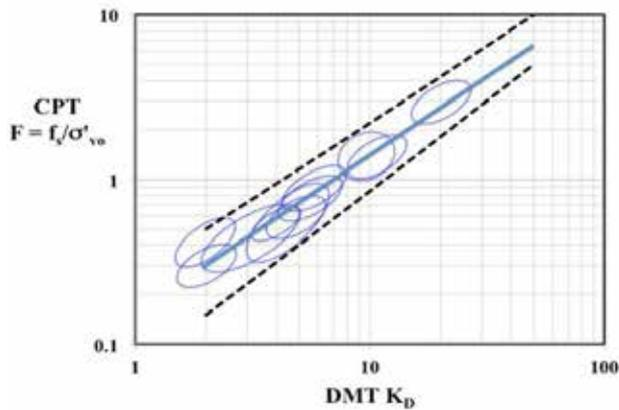
Figure 4. Relationship between DMT  $K_D$  and CPT normalized sleeve friction  $F = f_s/\sigma'_{v0}$  based on 10 sandy soil ( $I_c < 2.5$ ;  $I_D > 1.0$ ) around the world
