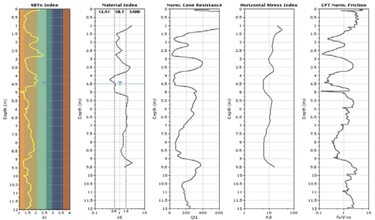
Figure 3. Comparison between CPT and DMT data in a sand site (Ledge Point) in Western Australia (data from Amoroso, 2011)
