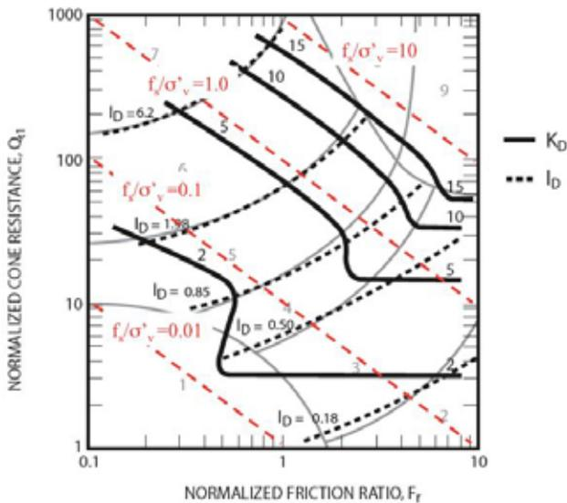
Figure 1. Approximate correlation between DMT  $K_D$  and  $I_D$  and CPT normalized parameters for soils with little or no microstructure (After Robertson, 2015)
