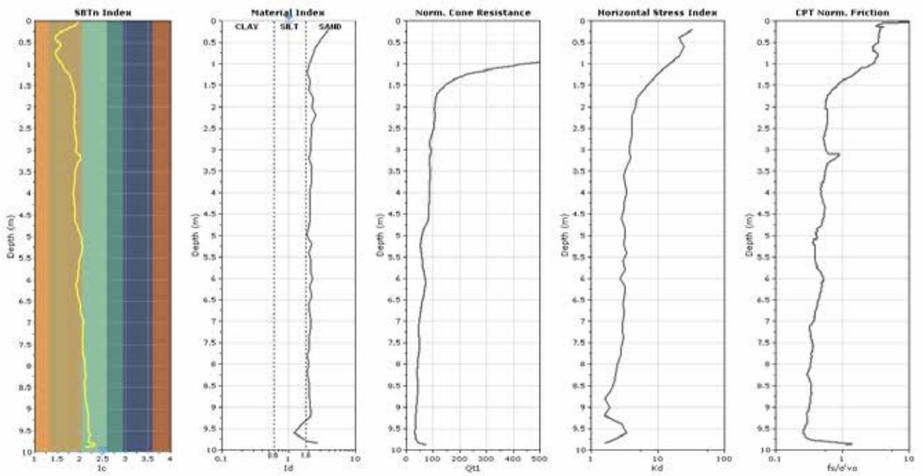
Figure 2. Comparison between CPT and DMT data in a sand site (Shenton Park) in Western Australia (data from Amoroso, 2011)
