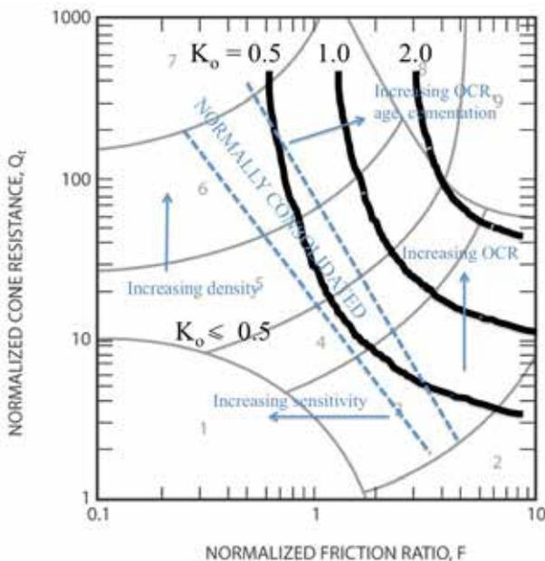
Figure 6. Suggested approximate contours of in-situ  $K_o$  on the CPT-based soil behavior type chart by Robertson (2009)
