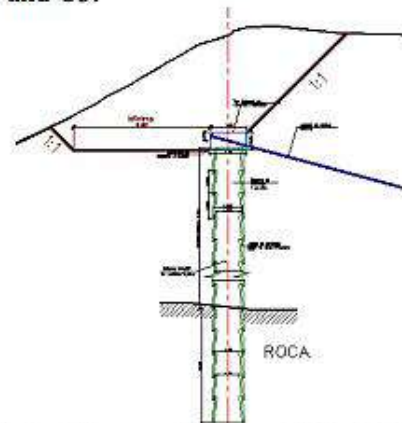
Figure 23- La Carbonera- Retaining Wall with Caissons
