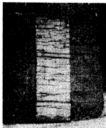
Fig. 3 Deformation of Paper Drains
